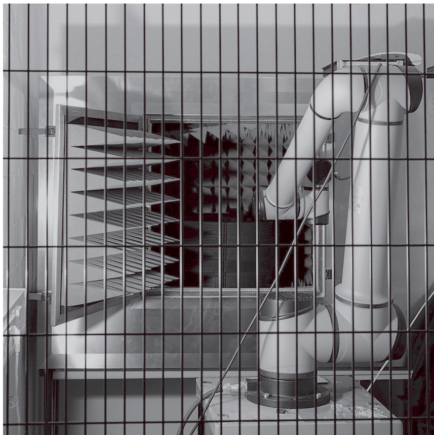
Figure 3. The Robot and RFID Measuring chamber are behind safety fences
