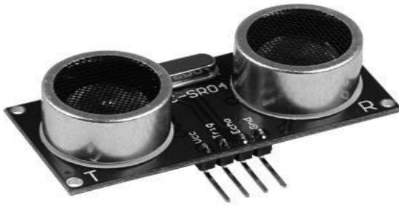
Figure 3 Example of an ultrasonic sensor
