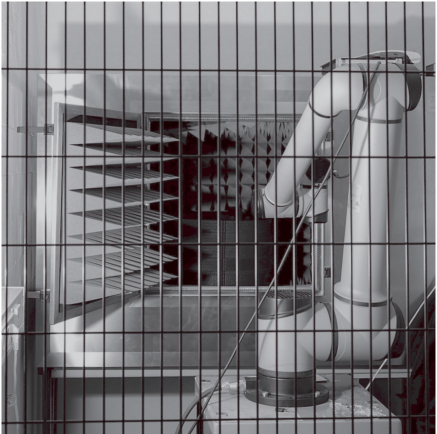
Figure 3. The Cobot and RFID Measuring chamber are behind safety fences
