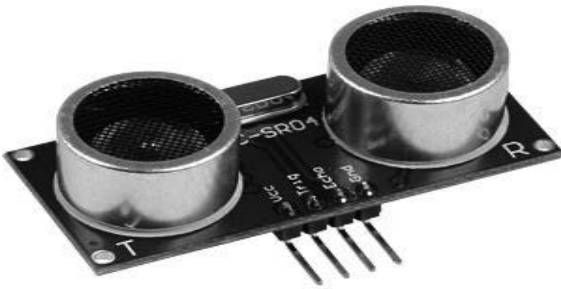
Figure 3 Example of an ultrasonic sensor
