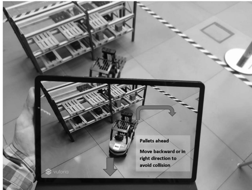
Figure 8 AR supported interaction and feedback GUI
