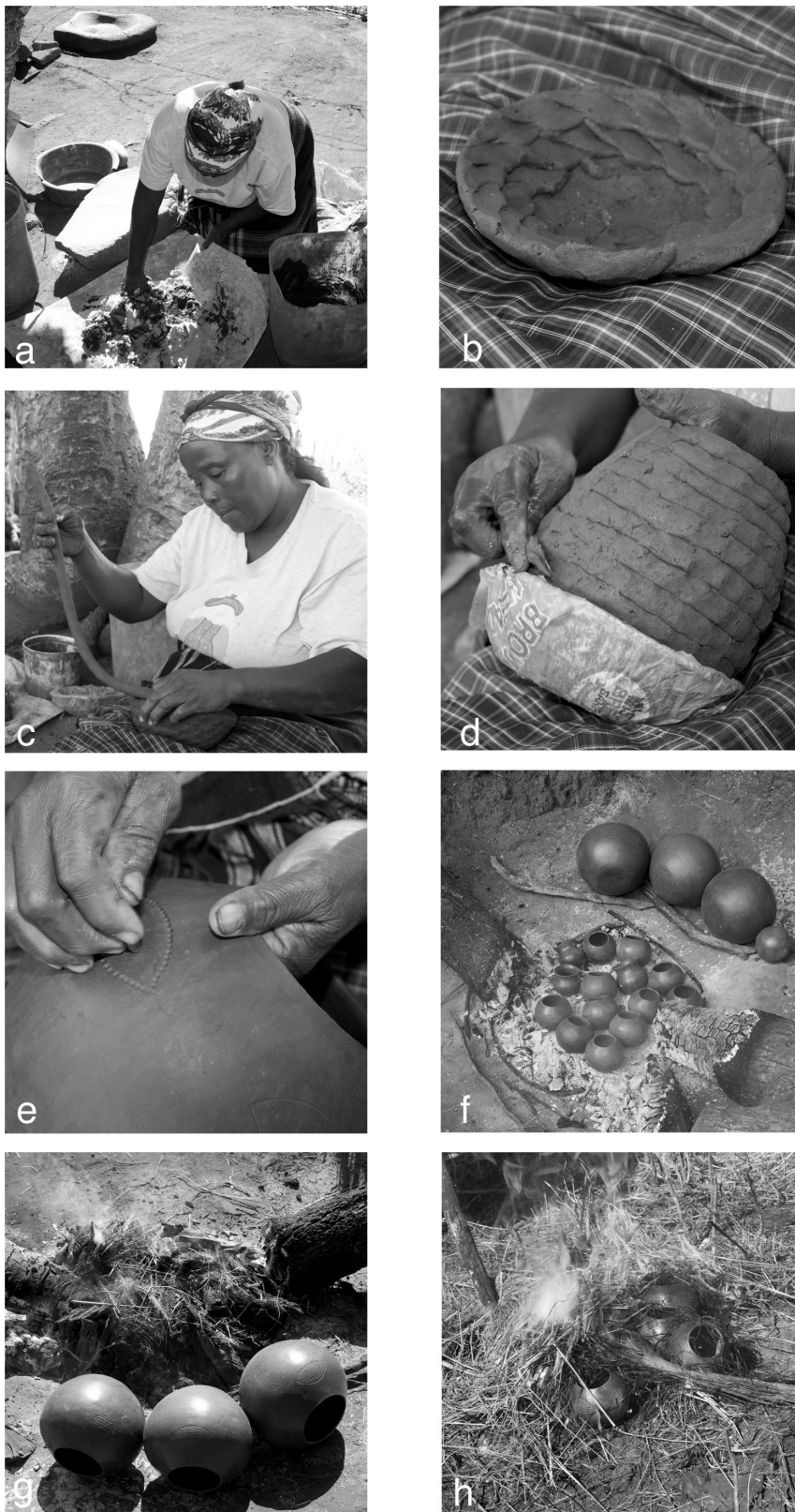
Fig. 2: Ceramic production demonstrated in the Manzini District: a) Mixing clays (clay soaking container to right and grindstone shown in background). b) Starting from a drawn clay disk. c) Coiling the roughout. d) Thinning and scraping the roughout in a support. e) Impressed decoration. f) Pre-firing using hard fuel. g) Firing using hard and soft fuel in the pit. h) Post-firing smoking of vessels in a mixture of green and dry grass.
