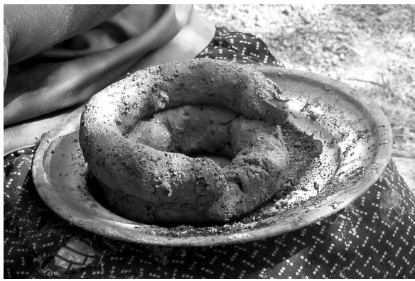
Fig. 13: Two coils are laid over the first ring to form a second one (LUB.01, Luba potter, Lubumbashi).
