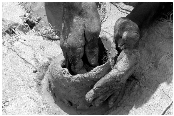
Fig. 7: Drawing of a ring (LUK.01, Bemba potter, Kawama). The potter sets a ring shaped lump of clay on the support. Having crushed downwards the outer part of the ring to fix it to the support, the potter inserts her hand inside the ring and draws the clay upward.
