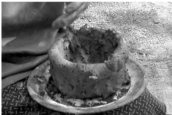
Fig. 14: The superimposed rings are drawn slightly upwards and outwards to give the rough-out a conical shape.
