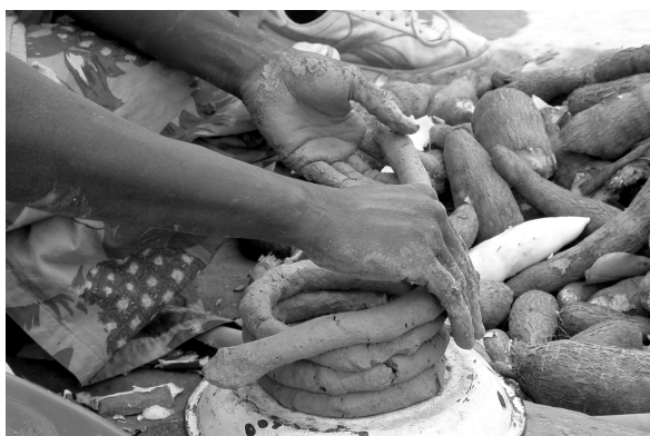
Fig. 2: Superimposition and pinching of “ring like” coils, or cylindrical coiling (NKO.01, Luba potter, Nkulu Majiba). Contrarily to spiral coiling, the roughing-out process starts with the belly of the vessel.
