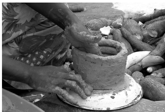
Fig. 3: The coil junctions are smoothed by drawing the clay downwards with the thumb (NKO.01, Luba potter, Nkulu Majiba).
