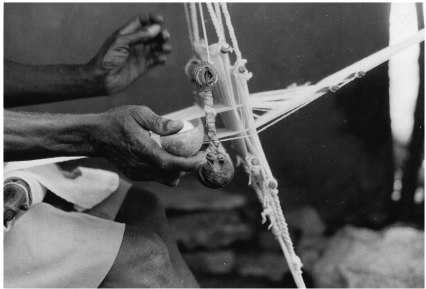
Fig. 7: Double-heddle loom (Bannani Kokoro, 1981): the breast beam, with its peg on the right hand side is in the foreground. Immediately in front of it are the beater and heddles, and beyond this is a double pattern stick (Photo: P. Lane).
