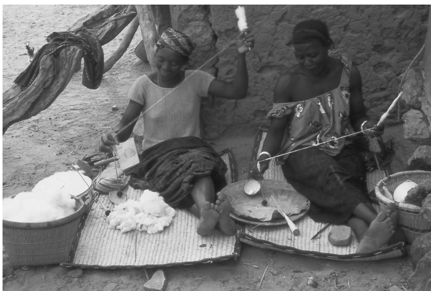
Fig. 1: Two Dogon co-wives spinning (Tasego, Séno-Gondo Plain, February 1983). The ginning stone and bar lies near the feet of the spinner on the right, and her ball of ash is in the small calabash just behind her leather-spinning mat. The woman on the left is holding her distaff in her left hand, and there is a pair of cards beside her on the right. The small tadu basket in the foreground contains unspun cotton waiting to be carded (Photo: P. Lane).
