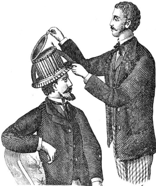
Figure 6: Measuring the Circumference of a Head with a »Conformateur« (taken from Möbius 1903: 17).
